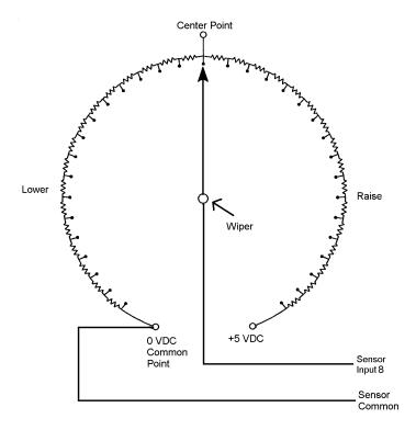
Figure 3-6: Typical OEM Potentiometer with 0 to +5 VDC Power
